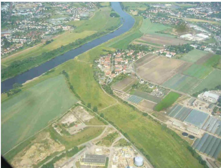
Figure 6.2 Levees at the floodplains of the Elbe river (federal waterway) and on both sides of the flood bypass channel downstream the city of Dresden at Kaditz Village in the centre of the picture (photograph: R. Pohl)
