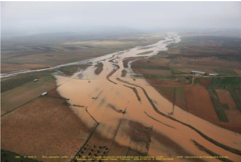
Figure 1: Aerial view of a flood event in Jabalón River (Guadiana basin). Existing levees were overflowed, what delayed the water drainage.
