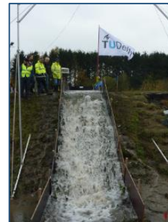
Physical breach modelling - the effects of wave overtopping on the landside slope of levees. Photo credit: TUDelft
